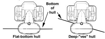
Align transducer centerline with hull bottom and attach to transom.
